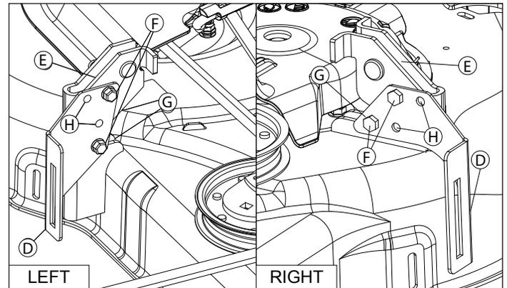
2. Connect brush support assembly to mower mount brackets at desired height (see page 4) using 3/8" x 3-1/2" Carriage Bolt (J), two Spacers (K), 3/8" Flat Washer (L), 3/8" Star Washer (M) and 3/8" Lock Knob (N). Thread 3/8" Lock Nut (P) onto the ends of the threads to prevent lock knobs from vibrating off.
