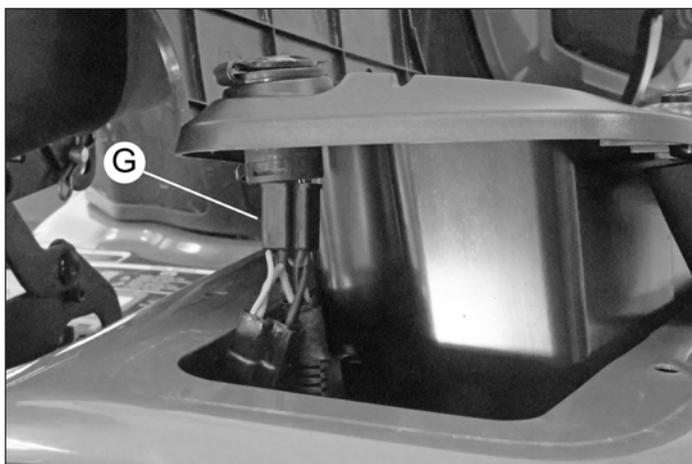
7. Reinstall the toolbox and tighten the M10 nuts on toolbox and the M13 nuts on the handle. Route the two connectors on the free end of the power harness through the elliptical hole in the frame (H) and secure
