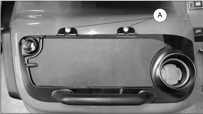
2. Locate the left support rib on the underside of the toolbox flange. Mark the top hole 3/8 in. to the right and 3/8 in. down. The bottom hole is 1-3/4 in. below the top hole. Drill a 7/16 in. hole at both locations.
