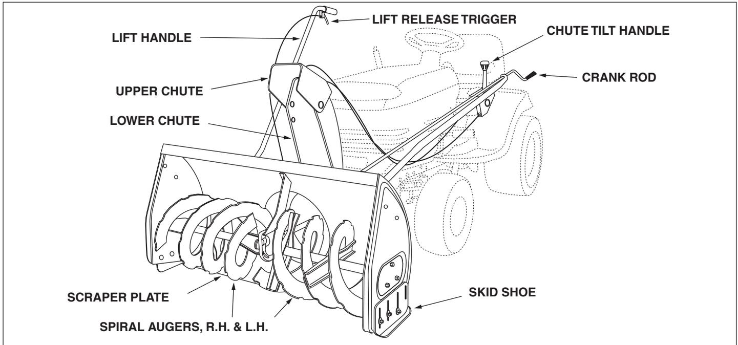
**CHUTE TILT HANDLE** Pivots the Upper Chute up or down to control the angle and distance of discharge.
