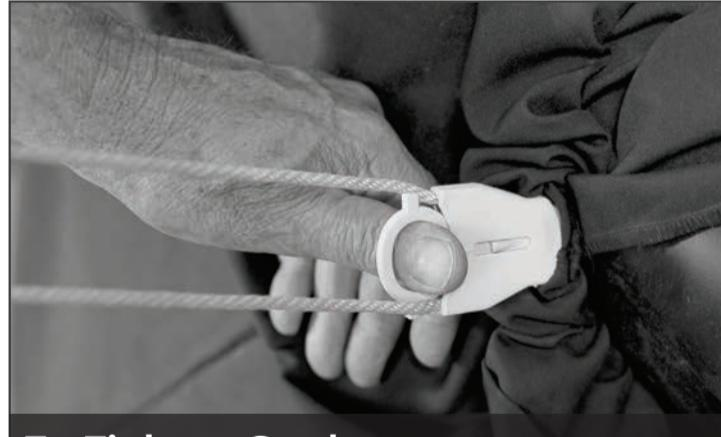
Push in on center loop of the cinching device and pull the end of the rope until taught.
