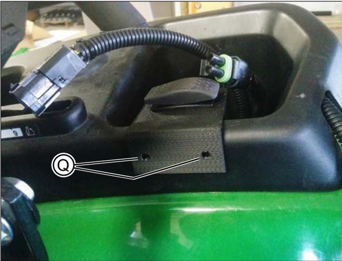
18. Connect the longer wire from the switch to the power plug and the short wire to the actuator on the TKV20.
