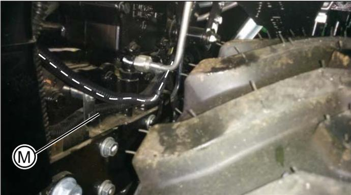
14. Working from the rear of the tractor, continue routing the wire harness up the ROPS and secure to the existing harness (N).
