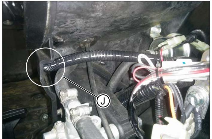
11. Looking at the side of the tractor, continue pulling the wire and thread it down through the hole next to the existing loomed harness (K). It is recommended to loop around the main tractor harness to prevent the wire harness from contacting the linkages.
