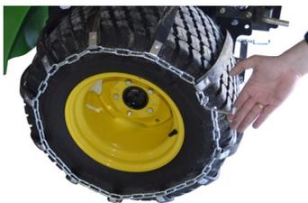
3) Latch Operation: Insert the top of the latch through the selected link.
