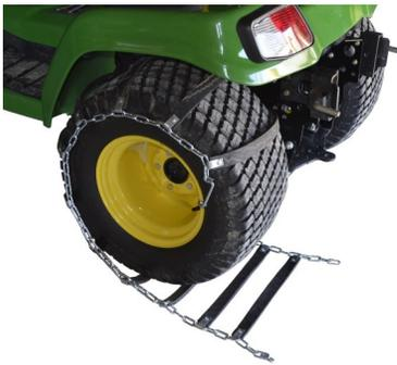
2) Drive onto the tire chains leaving approx. 2/3 of the chain in front of the tire and drape the long portion of the chain around the tire. Hook the inside first, starting with the very last link. Repeat with the latch side (outside).
