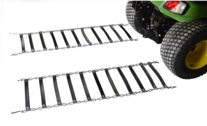
1) Lay the tire chains out on the floor behind or in front of the rear tires of the vehicle, with the peened side of the rivets up (head down). The hook goes to the inside and the latch to the outside of the tire.
