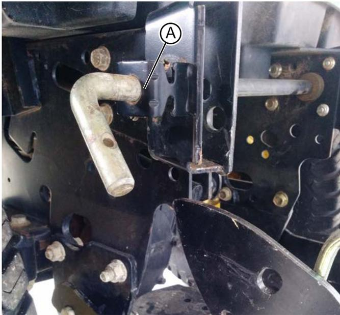
4. Pull locking pins (A) outward and rotate to the locked out position.
