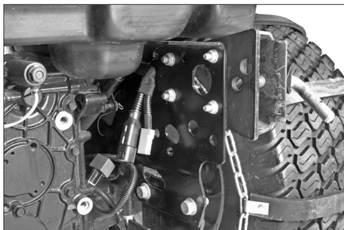
8. Attach the display harness (J) to the connector on the rear of the display (K).
