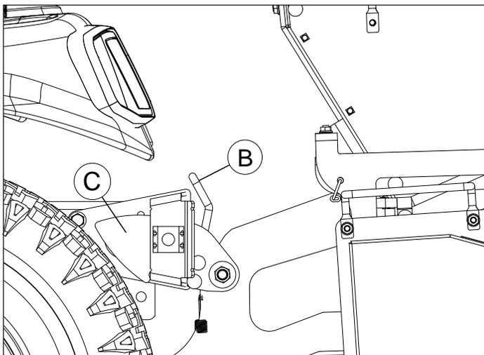
5. Lift the spreader slightly and pull rearward on the upper cross rod (B) to disengage the lock arms (C) and lower the spreader to the ground.
