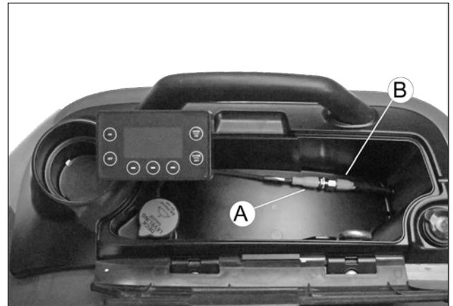
2. Remove display by sliding bracket out of mount inside toolbox.
