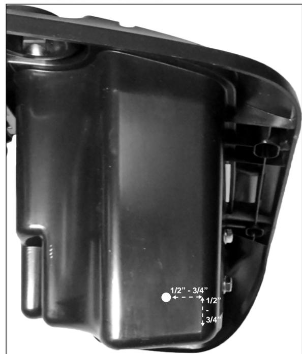
5. Install grommet over circular connector on the power harness (D) and feed harness through the hole in the rear of the tool box seating the grommet in the hole.
