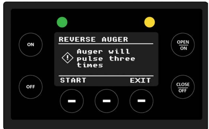
3. If the auger needs to be reversed further, press start again and wait for the reverse cycle to complete.
