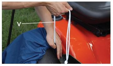
12. Hang Leaf Bag on S-hook (W) using Grommet. To prevent interference and tangling, hook the drawstring (X) onto the S-hook.
