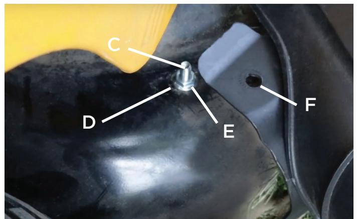
3. Slip the rear hole (F) in the chute over the bolt installed in step 2.
