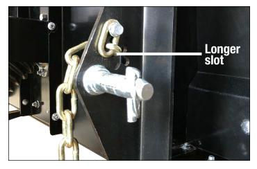
2. At the rear of the tractor, remove the two bolts from the existing metal plate. Remove the metal plate and install the Chain Connection Plate (B) as shown, using the 5/16" Flange Bolts and 5/16" Flange Nuts. Repeat on the other side of the tractor.
