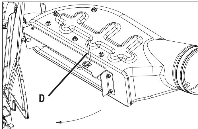
4. With boot against mower deck, lower handle (E) rearward to secure boot (shown with no discharge chute for clarity).
