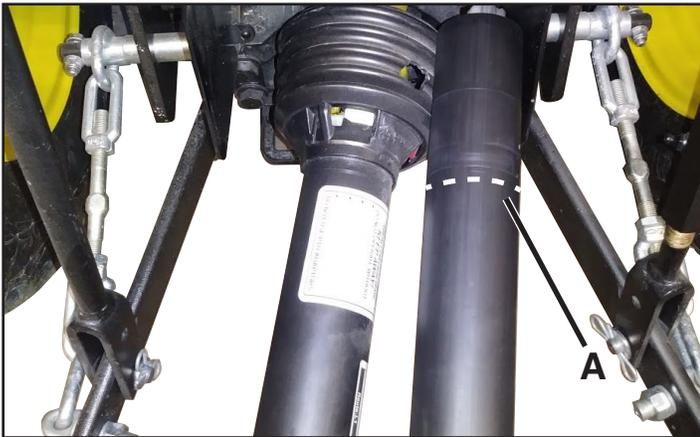
3. Remove both halves of the PTO shaft. Cut the guard an additional 1.25 - 1.5 inches than the amount measured or marked.
