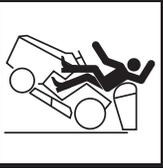
To avoid injury, install front ballast per operator's manual.
